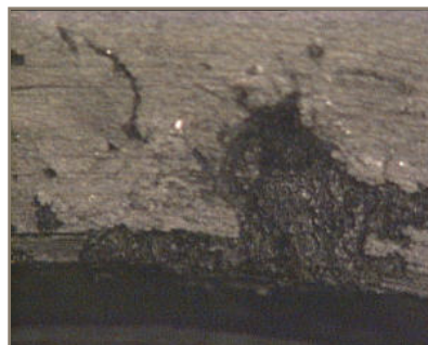
Pitting on filter end-cap
