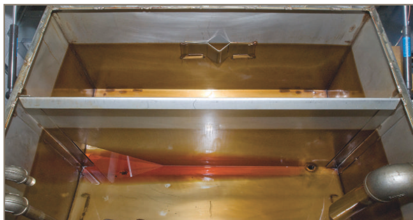
Varnish is attracted to metal surfaces, this results in an overall decrease in productivity.
